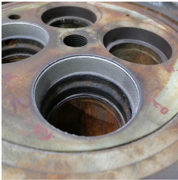
CLADDING OF AUX.ENG CYL HEAD VALVE SEAT POCKET
