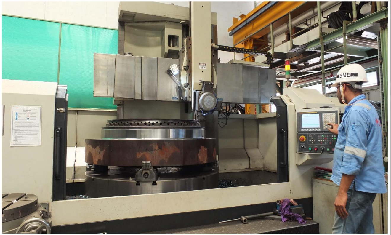
CNC FINAL MACHINING OF CYLINDER COVER
