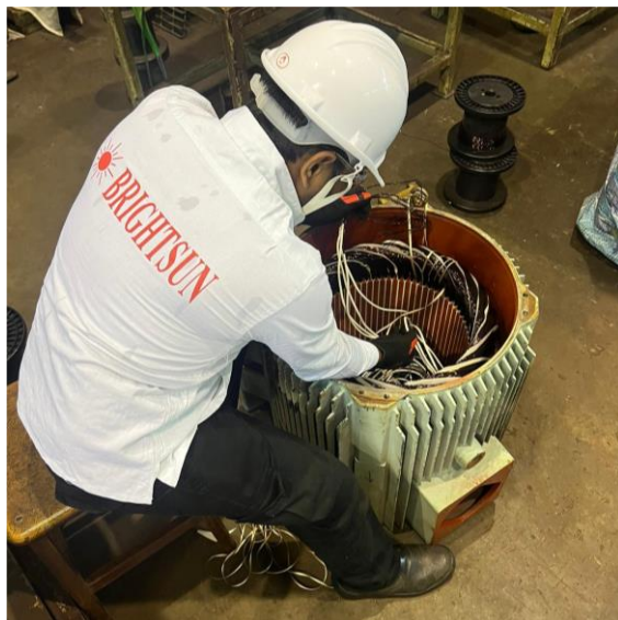
REWINDING OF ELECTRICAL MOTORS
