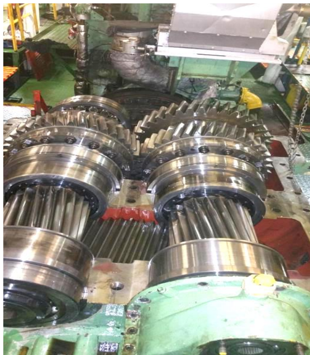
GEAR BOX OVERHAULING
