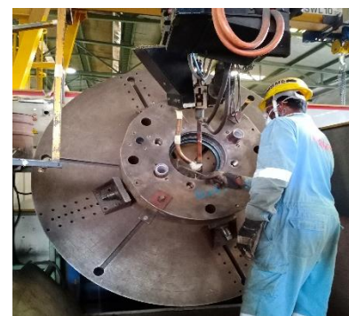
RECONDITIONING OF CYLINDER COVER
