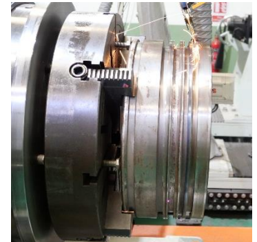
CLADDING OF PISTON RING GROOVE
