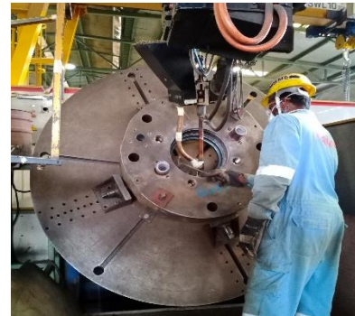
RECONDITIONING OF CYLINDER COVER
