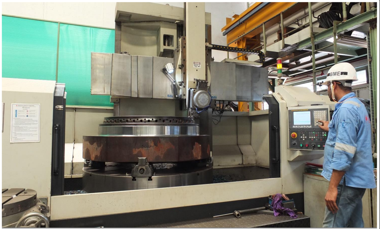
CNC FINAL MACHINING OF CYLINDER COVER
