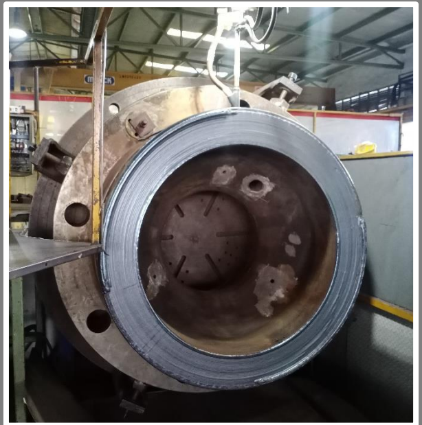
AUTOMATED SAW WELDING OF CYLINDER COVER
