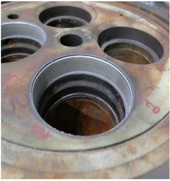
CLADDING OF AUX.ENG CYL HEAD VALVE SEAT POCKET
