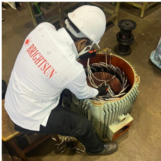
REWINDING OF ELECTRICAL MOTORS
